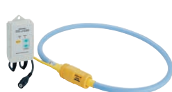
FLEXIBLE CLAMP-ON SENSOR 9667 Current up to 5000A AC Diameter up to 254mm Rogowski-type current sensor
