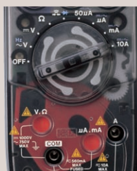
10A range Only A and COM terminals open
