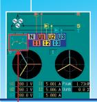
Use the wiring map, vector map and data monitor to check for proper wiring before taking measurements - don't miss out on important power data just because of minor wiring mistakes!
