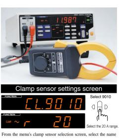
of the sensor with the cursor key and press the **ENT** key. Then, select the same range as you set for the sensor with the cursor key.
