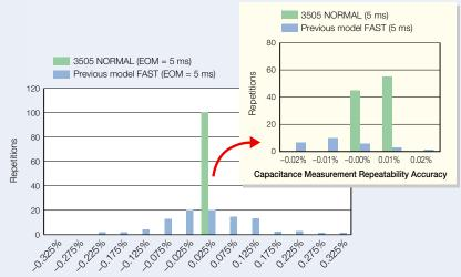
Capacitance Measurement Repeatability Accuracy Measuring 1 pF (at 1 MHz, 1 V)
