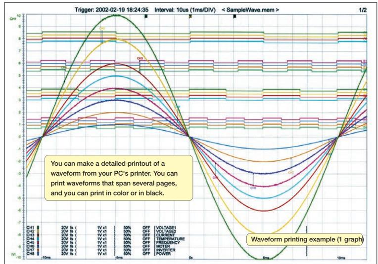
When a waveform is displayed on the screen, you can copy that waveform to the Windows clipboard, or make a hardcopy of the waveform. You can also paste the waveform into text, as well as associate the waveform with whatever application you want to start when you open that waveform.
