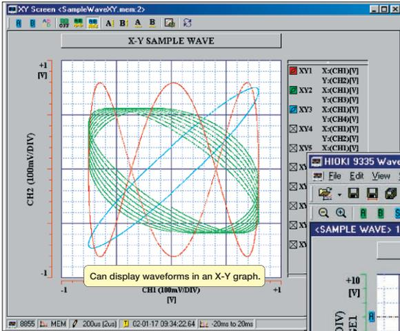
The 9335 lets you load binary files from a MEMORY HiCORDER and then check the waveform or measured results on the Waveform Display Screen and the Numeric Display Screen. The 9335 also supports the memory recorder function X-Y display. The Waveform Display Screen and the X-Y Display Screen also can be split into graphs for each channel.
