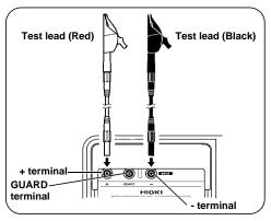
4. Clip the ends of the test leads to the circuit to be tested. When the voltage exceeds 50 V, the mark and key lamp blink.
