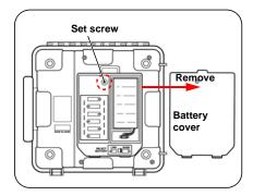
Place six LR6 alkaline batteries into the battery compartment. (Replace all six at the same time)
