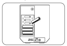
Turn the battery selector switch to LR6.
