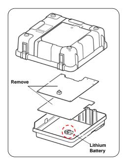
The battery is located on the remaining PCB as shown in the illustration on the previous page.
