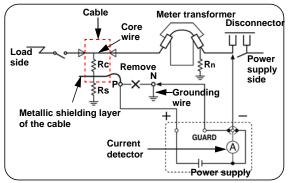
Rc: Insulation resistance of the insulating material of the high-voltage cable (Between core and metallic shielding layer)
