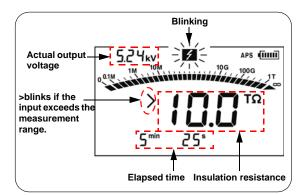
If > blinks, the input value is out of measurement range. Example: >  $10.0 \text{ T}\Omega$  means "larger than  $10.0 \text{ T}\Omega$ ."
