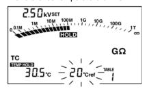
Adjust the reference temperature using the key.
