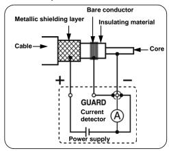
When testing the insulation of a cable, as shown in the diagram above, wind a bare conductor around the surface of the insulating material and connect the conductor to the GUARD terminal. This prevents the leakage current on the surface of the insulating material flowing into the current detector, which enables the actual resistance of the entire volume of the insulating material to be measured.
