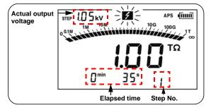
The test voltage rises at regular intervals and the test stops automatically.
