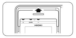
Connect the red test lead to the + terminal and the black test lead to the - terminal. Connect the blue test lead to the GUARD terminal if necessary. Fully insert the test leads. See 3.2.7 "Use of GUARD Terminal" (page 77).
