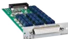
MULTIPLEXER UNIT Z3003
